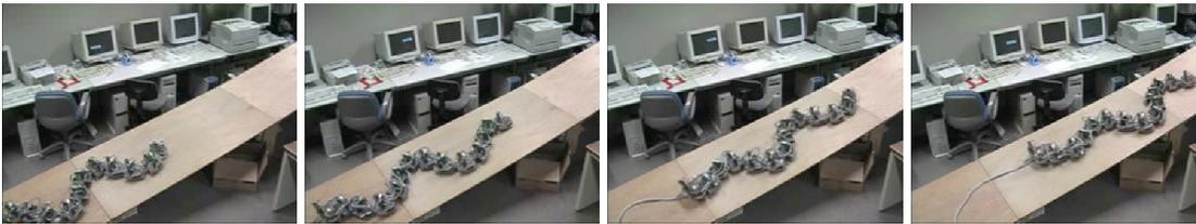
Fig. 6.14: Experiment to show creeping locomotion on a 10[deg] slope (Unsymmetric case)
