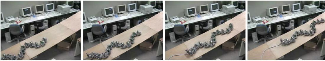
Fig. 6.13: Experiment to show creeping locomotion on a 10[deg] slope (Symmetric case)
